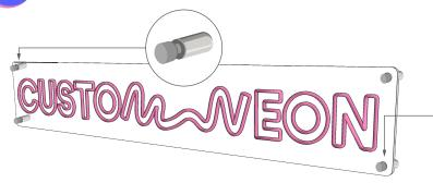
STANDARD MOUNTING KIT ALLOWS THE SIGN TO SIT 2.5cm OR 1" OFF THE WALL.
