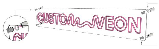
4. JELLY WASHER TO BE PLACED ON TOP OF EACH SPACER AND HOLES IN ACRYLIC SIGN LINED UP WITH SPACER BEHIND SIGN.
